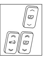
The sunroof/sunshade switches are located in the headliner between the driver and front passenger. One switch operates the front sunroof and another switch operates the front sunshade. The third switch is for the rear sunshade.
